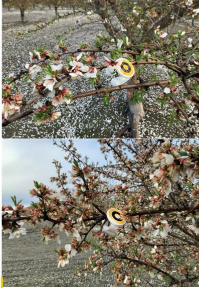
Figure 5: Acoustic sensors used to track in-field pollination visits.
