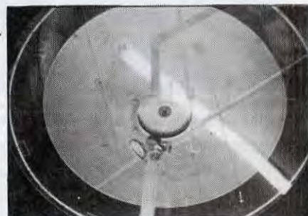
The top of the Cook & Beals Spin Flow cappings separator. The machine has a clear plastic cover (note light reflection) so operator can observe cycle.
