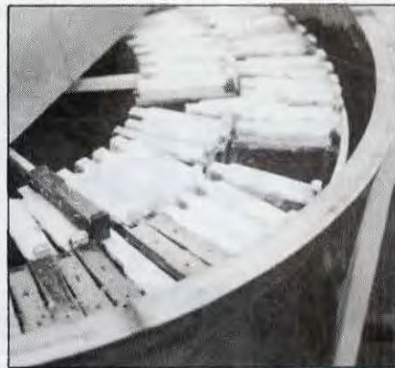
A loaded extractor. The Kerr's use two — one can be down being unloaded and then loaded while the other is running.
