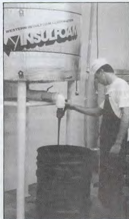
Extracted honey eventually ends up in one of the storage tanks. These are insulated with two layers of 1/2" foil-backed insulation and kept just warm enough to keep honey flowing.
