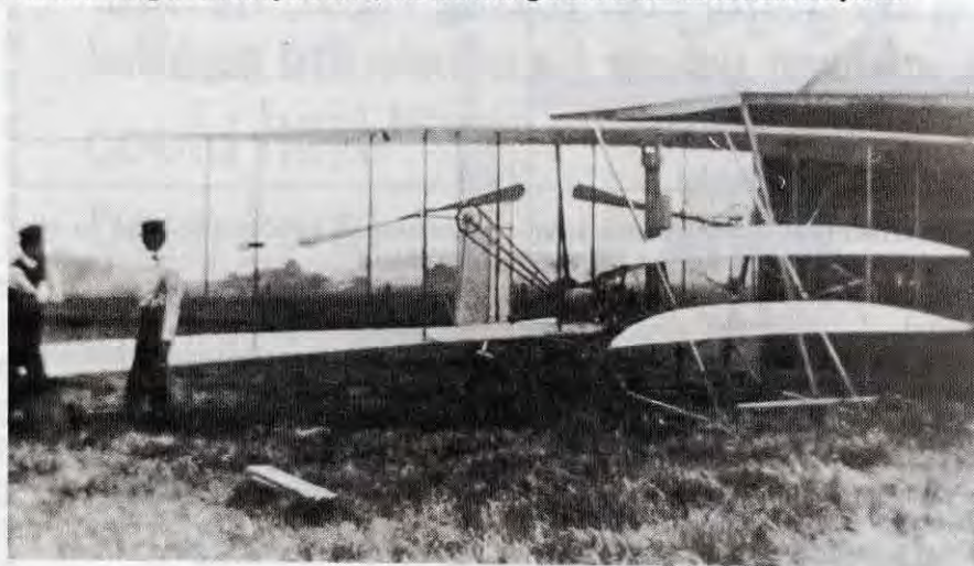
Orville (left) & Wilbur at Huffman's Prairie, May, 1904. The 'Flying Machine' slides into the little 'hangar' sideways. Part of the launching track is visible beneath the plane.
