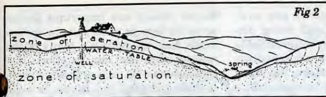
Water percolates into the soil by gravity. The water table level, when examined in a closer view shows seasonal fluctuations. "Geomorphology" A. K. Lobeck, McGraw Hill, NY 1st ed. 1939.
