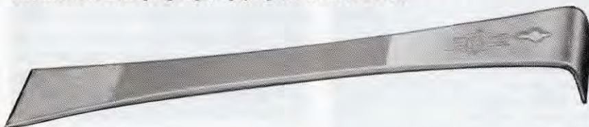
Hive tools also are available in several sizes and shapes. This is the most commonly used model. It has a scraping edge, a prying end a rail remover.
