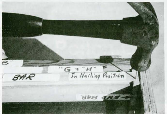
Attaching the bottom bar. Note how the frame fits flush with the bottom of jig. This would work equally well with split bottom bars.
