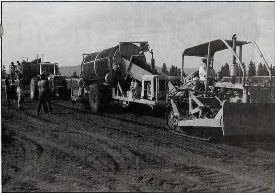
Strawberry plant harvest. The revolving drum shakes the soil from the roots of the plants, but doesn't damage the crown.
