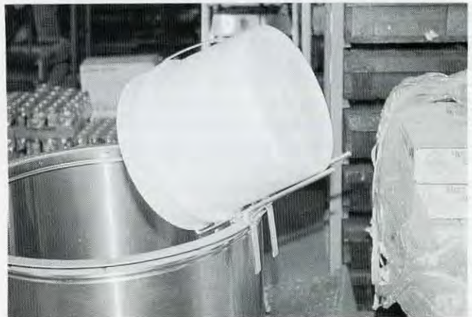
Maxant's newest Beekeeper's Helper. A holder for five-gallon pails that fit a variety of tanks.
