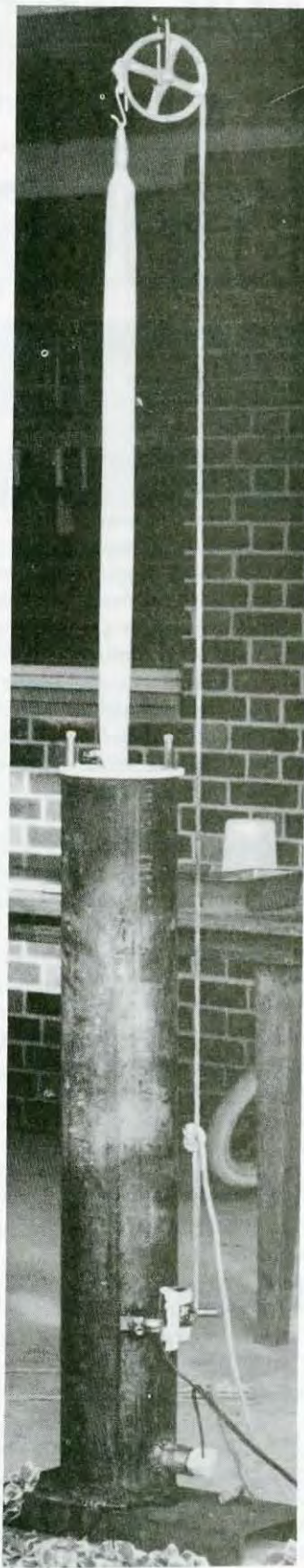
The dipping process is simplified by using a pulley instead of standing on a chair. After several dips the candle has to be reversed so it doesn't become tapered. After it reaches an inch and a half quit for a day to let it cool.
