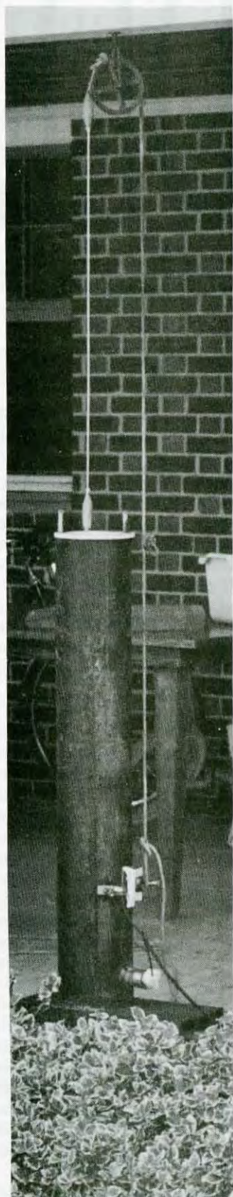
The dipping process is simplified by using a pulley instead of standing on a chair. After several dips the candle has to be reversed so it doesn't become tapered. After it reaches an inch and a half quit for a day to let it cool.
