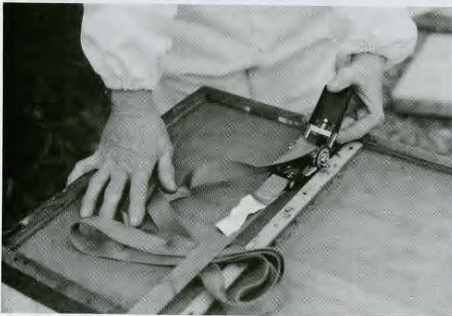
Showing detail of ratchet mechanism on belt and double screen.
