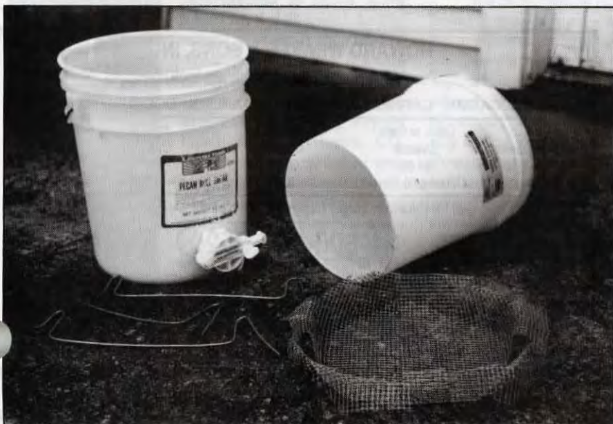
One pail with gate attached (L), one with bottom removed (R), a mesh 'hat' and three wire supports.
