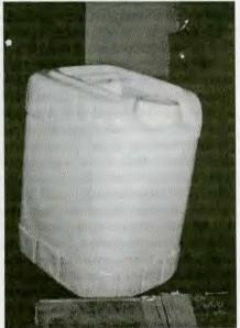
The five-gallon containers used at Draper's is a square pail, stackable with a recessed handle. The spout fits the commonly available plastic gates.
