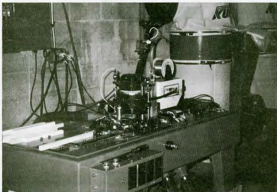
The machine developed by Robert Koehnens that makes the mini-queen cage. It can produce 6,000/day.
