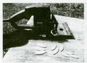
The biscuit slot cutting tool is shown with three each of the three standardized sizes of biscuits. Left: size  $#20 (24 \times 58 \text{mm})$ ; center: size  $#10 (20 \times 52 \text{mm})$ ; right: size  $#0 (16 \times 47 \text{mm})$ .
