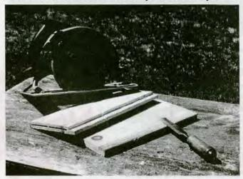
To form the rabbet for frame rest on end boards, multiple saw cuts kerfed out most of the wood to the appropriate width and to 1/2 the board thickness. The remaining wood was easily removed with a chisel or utility knife.
