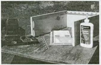
Medium depth super ready to glue up shown with biscuit slot cutting tool, frame spacers and glue.
