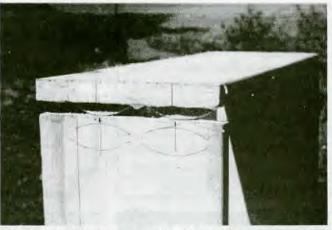
With biscuits and glue in place this side board is ready to secure to the end board. The centerline marks on each biscuit location on boards to be joined are a key measurement although biscuits and slots do allow some room for fine tuning adjustment.
