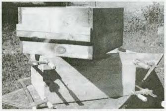
A finished hive body showing hand lifting bars on recently clamped hive body. The finished box on top was made last Winter and left exposed to the elements inside and out for six months to test whether the corners would open up. They did not.
