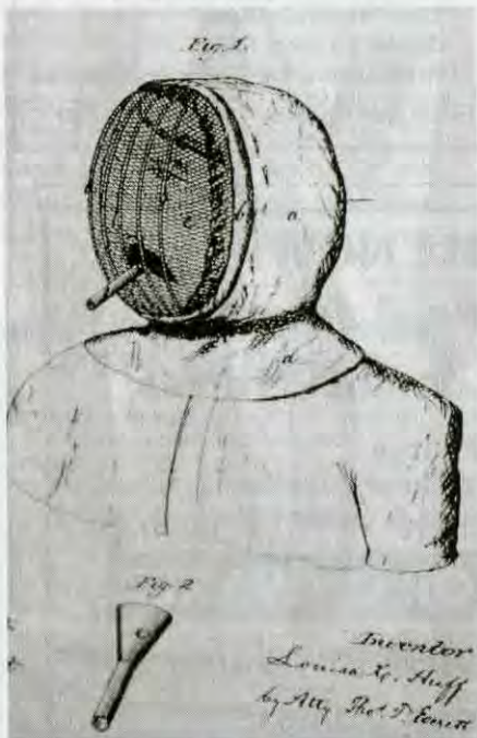
An 1873 patented mask for protecting beekeepers. The pipe was used to blow smoke on the colony.
