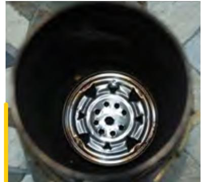
Figure 10. Insert your improvised aerator support first, legs down. Having a gap between the rim of the improvised support and the smoker walls only adds to the air flow. That's a good thing.
