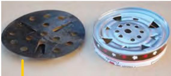
Figure 5. I ended up adding holes with a drill, so to come closer to the original aeration volume found on the original aerator piece. It has 13 holes plus the tabs when pulled down. Considering structural integrity of the can, I ended up with 17 holes. We are not quite done here...
