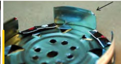
Figure 7. Notice how all cut metal is folded in some fashion to help prevent accidental nicks and cuts. The corners of the leg were also bent to add structural strength to safety.
