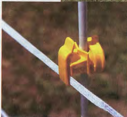
Keep the wire to the outside for strength.
