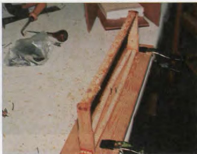
Frame formed parallel to board. Note wide space for inserting wax foundation.
