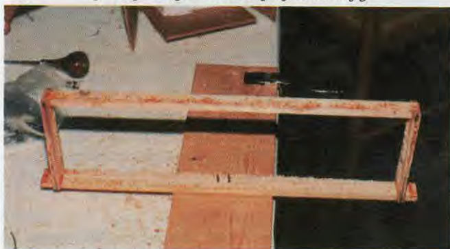
Split top bar placed on top of nails in jig.
