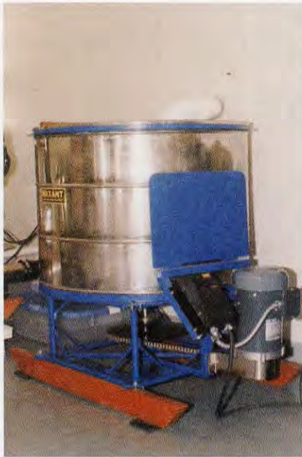
Rebuilt maxant cappings spinner w/ variable speed DC motor (facilitates easier cappings removal & greater honey/wax separation). PVC pipe top loads, honey drains back to clarifier.
