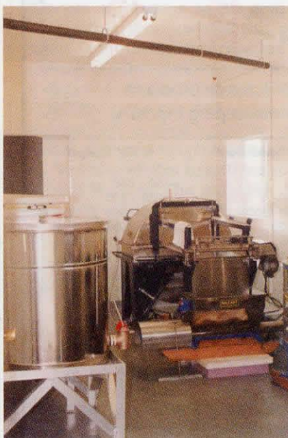
General view of extracting set-up: Spinner, far right, Cowen 18 frame extractor w/Maxant auger, front. Overhead, black insulated pipe runs from honey pump to storage/bottling tanks, left in picture.
