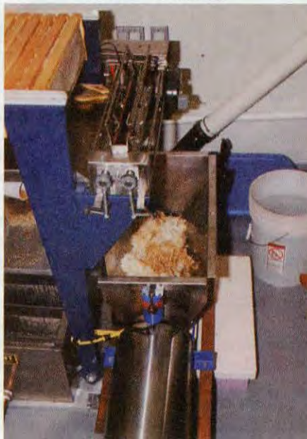
Detail of uncapper, auger below, and feed pipe rear to spinner.
