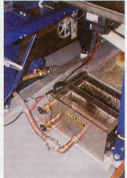
15 gallon Maxant clarifier extractor, left and spinner, right (out of picture) drain through screen. Note quick-connect "c lock" on hose which facilitates cleaning.
