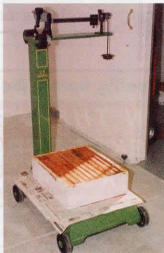
Incoming supers and filled containers are weighed on a 50-year-old rebuild platform scale.
