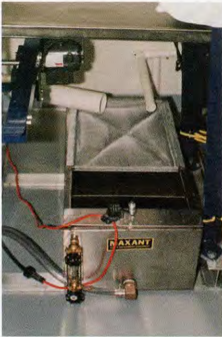
15 gallon Maxant clarifier. . . Extractor, right, spinner, left drain through screen. (Float switch on front of tank.)
