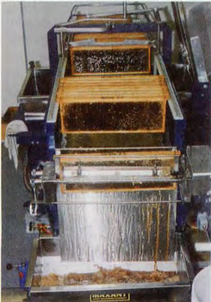
Loading & unloading extractor (done in one motion). Uncapper, front (cappings fall into auger below) 18 frames in, 18 frames out.
