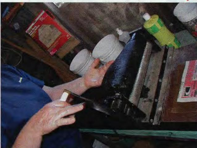
The wax, enclosed in the thin plastic is then rolled through the mill. These hand-cranked rollers are specially made by Tom Industries of Yuma to produce a cell that measures just under 4.9 mm. Joe and I later met Tom on our way west, and saw his shop. The newspaper pieces shown are used to separate the fresh sheets of foundation to prevent their sticking together.
