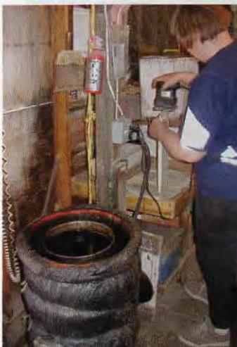
*Before beginning work for the day, Dee sands all surfaces of the wooden dipping blank to ensure water will adhere to it. When dipping, the wax sheets peel off easily if the wood is wet. Wax for foundation making is melted in the dipping tank (left foreground). The tank is insulated, water jacketed, electrically heated, and thermostatically controlled.*
