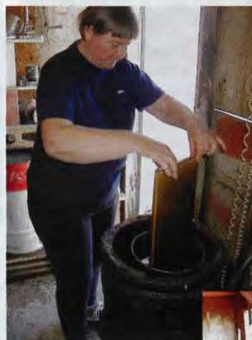
*Dee dips the blank completely into the molten wax twice, once with each end down, to ensure an even, thick coating. She waits a moment between dips to allow the wax to set a bit. The wax for dipping is held just above the melting point, so it makes a thick coat and cools quickly.*
