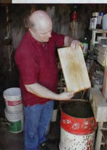
*Joe examines the blank as he prepares to dip it into the water tank. Water ensures the wax will peel off cleanly, and the blank is dipped into water before each new sheet is made.*
