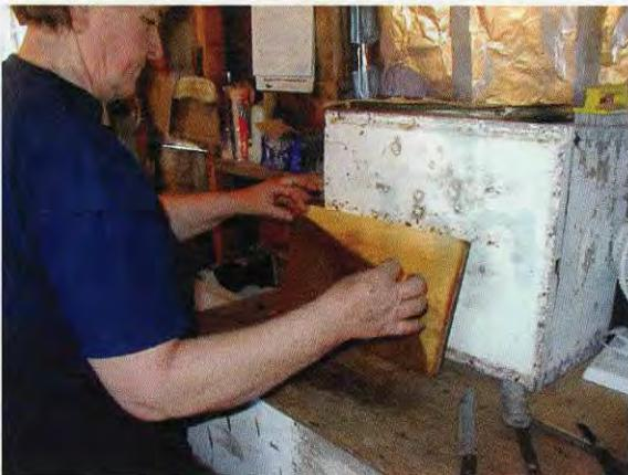
While still soft, two blank sheets of wax are peeled off the damp board - one from the front and one from the back — and stacked awaiting milling. Scraps go back into the melting tank.
