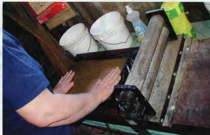
The still-blank wax sheet is wetted with water and a biodegradable dish detergent to prevent sticking and sandwiched between two layers of plastic garbage bag in preparation for a trip through the mill.
