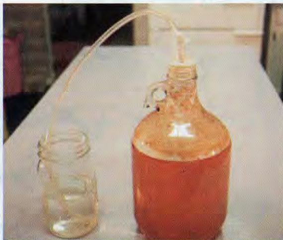
A fermentation rig. Plastic wrap keeps things clean. Note the placement of the stopper and the hose.
