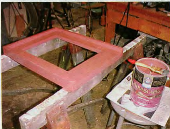
The scraped and painted rejuvenated bottomboard.
