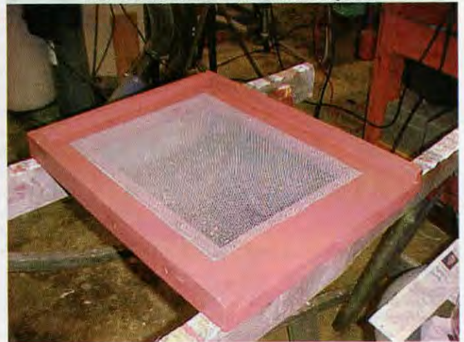
The 1/8" hardware cloth screwed in place.
