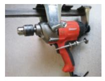
**Note:** The drill used for this article and the subsequent extractor motorization is a ½" – zero to 600 RPM variable speed drill.
