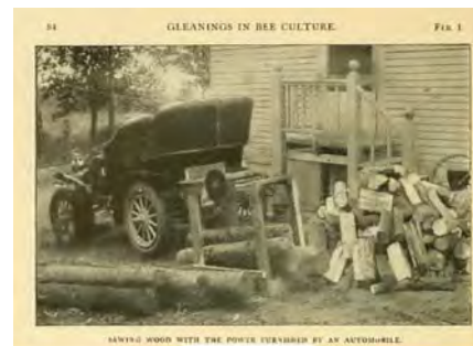
SAVING WOOD WITH THE POWER FURNISHED BY AN AUTOMOBILE. Feb. 1, 1909 Gleanings
