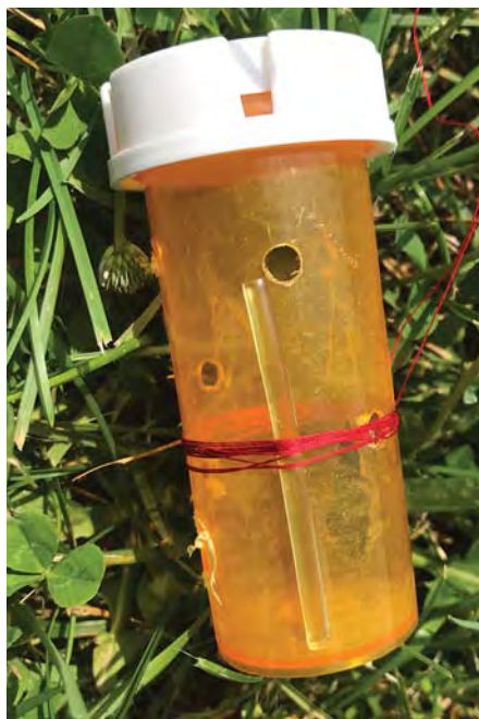
Drone Lure: The lure is a pill bottle with holes drilled into it. There is an artificial queen pheromone stick inside the bottle. The lure hangs on a thread about 20 feet below the flying UAV.
