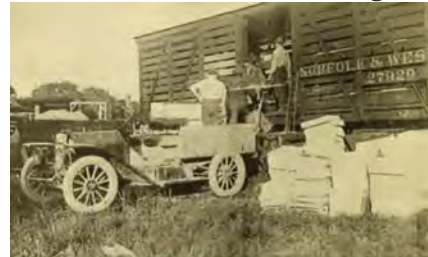
Unloading bees from box car. Picture from July 15, 1915 Gleanings. Truck body placed on old touring car.
