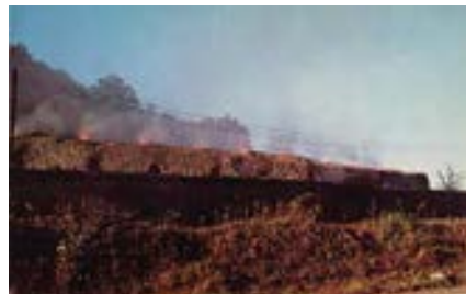
Beehive Coke Ovens, Norton, Virginia – one of the oldest methods of manufacturing coke from coal. Wise County is one of the few places in the U.S. where such ovens may still be seen.
